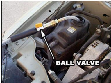
3. Turn Right Dial to "Vacuum/Drain Waste" position.
