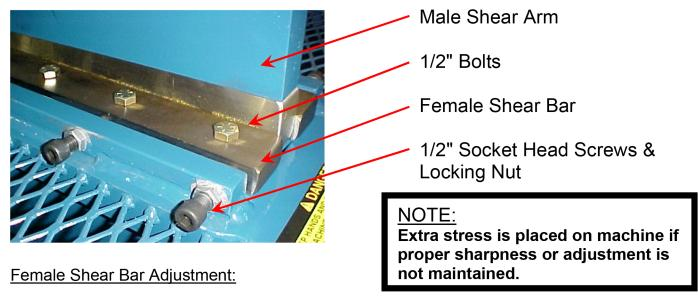
As the steel belting from a tire starts to string out and not cut properly the original bar edges will eventually need to be adjusted.
