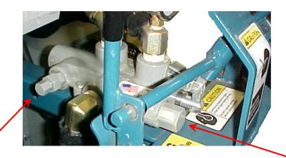
If valve "kicks out" on the shear arm return stoke, the detent will have to be slightly tightened. Tighten outer nut 1/4 turn and tighten lock nut. Continue to cut. If valve still "kicks out" readjust it another 1/4 turn.
