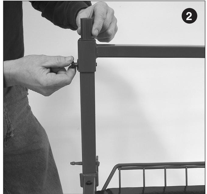
Insert RO Bracket (P/N 290-40) into upper frame support. Reinstall 3/8" hex bolt and tighten.
