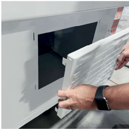
Designed with a Post exhaust filter for a cleaner environment in the work area
