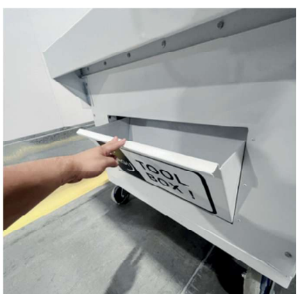
Design with a tool storage box to maximize work space in the down draft table
