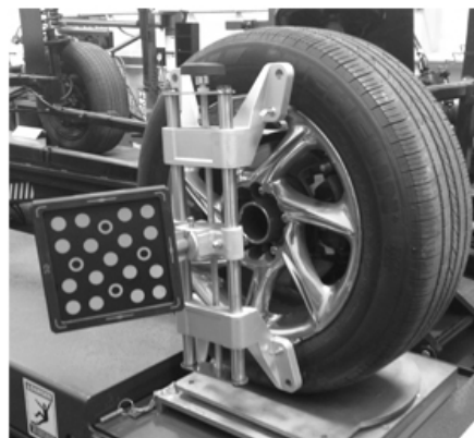
FRONT TARGET INSTALLATION
