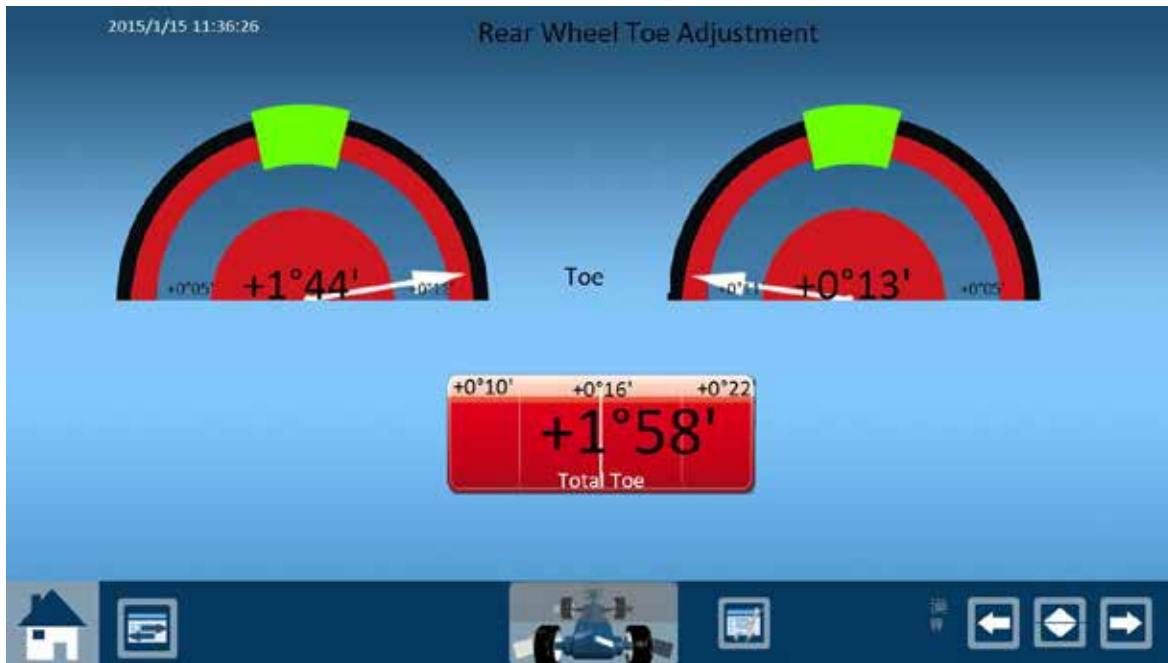
Individual adjustment of rear wheel Toe
