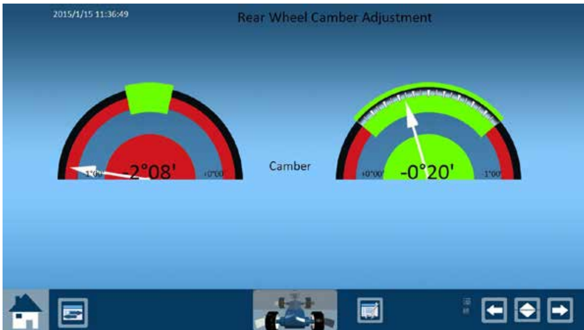
Individual adjustment of rear wheel Camber
