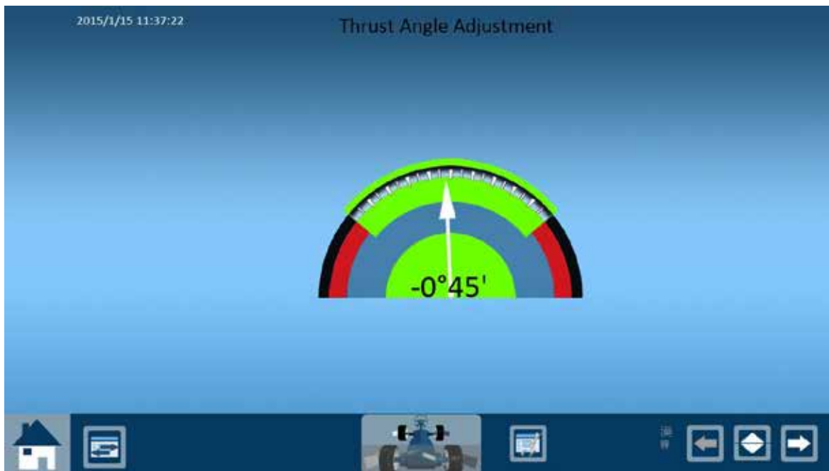
Individual adjustment of rear wheel thrust angle
