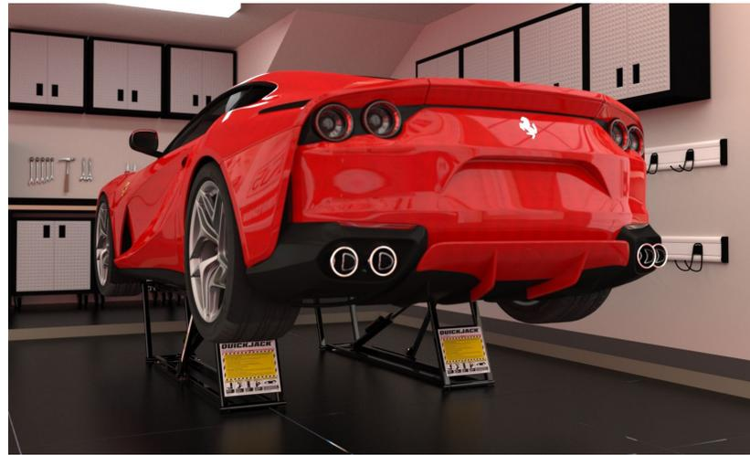
QuickJack handles the lifting and safe-keeping of your vehicle with the simple push of a button, and there are no crossbeams on the ground to get in your way. Each of the two frames feature automatic locking bars that are essentially “jack stands” built right into the sides.
