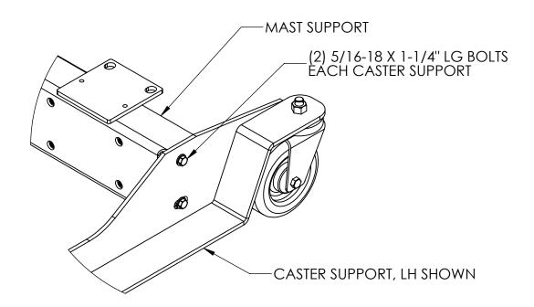
1. ATTACH CASTER SUPPORTS RH & LH TO MAST SUPPORT USING HARDWARE NOTED
