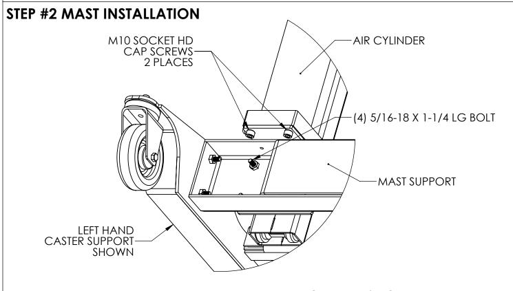
ATTACH THE MAST TO THE MAST SUPPORT USING HARDWARE NOTED
