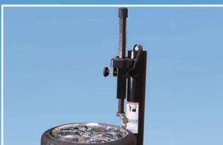
An unobtrusive, vertical design, column-integrated air tank helps conserve valuable shop space with a large volume for increased blasting capabilities.
