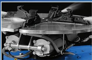
A direct burst of compressed air comes through the clamping jaws to facilitate bead seating.
