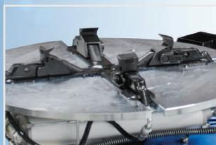
To safeguard the wheel's integrity, these nylon-covered jaws are self-centering and grip the wheel firmly for elevated stability and safety.
