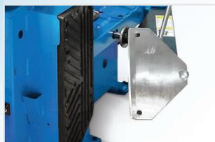
A conventional side-shovel bead breaker, featuring an ergonomically positioned pedal control situated a small distance from the shovel, is the quickest solution for efficiently handling a range of tires.
