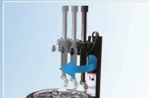
Optimization of space is skillfully ensured with a mounting arm that pivots to the side, allowing the machine to be efficiently installed directly adjacent to a wall.
