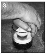
Place the Handy Packer on a flat, solid surface and press down on the cap until the old grease is forced out and new grease shows on top of the bearing.
