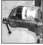
The Handy Packer can be used in a vise with heavy grease. The ribs on the bottom of the cup fit on each side of most vise jaws to hold the cup in place when tightening.
