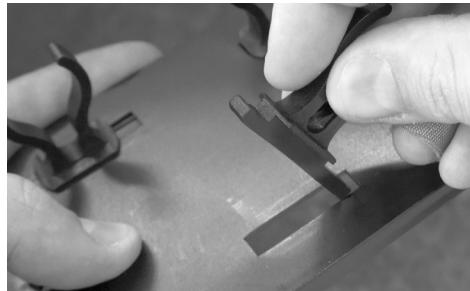
Slide long end of clip through the top of the holder, away from the small detent (A).
