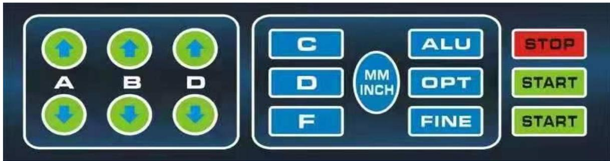
(A) A = Distance of machine to wheel. Manually enter the reference distance size with button A, press the arrow to go up, increase the input size, press the arrow to go down, reduce the input size.
