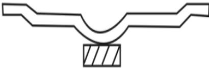
Static Balancing- Static balance correction is performed on one side of the tire. This consists of only one side or single weight placed on the rim. (one clip on or adhesive weight)
