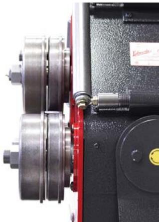
With the roller dies configured to the material, tighten the dies onto the drive and idler shafts with the wrench provided. **DO NOT OVERTIGHTEN SECURING NUTS TO SHAFTING.**
