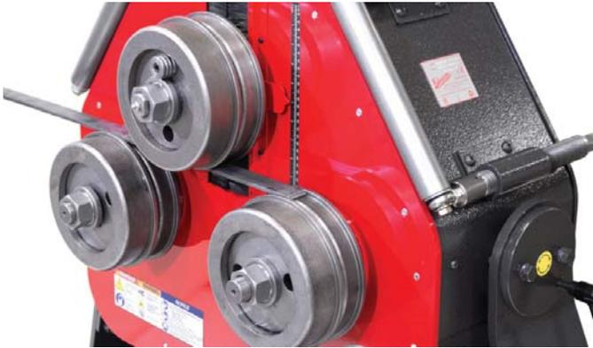
Adjust the pressure roll to capture the material being roll formed by nesting the roll set and spacer.
