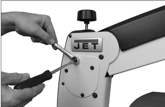
Figure 9-12: tightening arm lift
