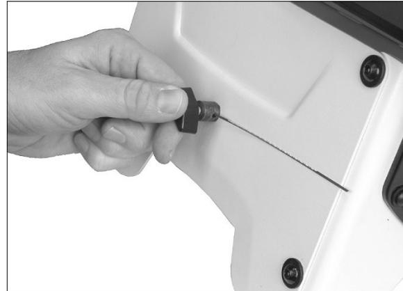
Figure 9-2: installing blade into holder
