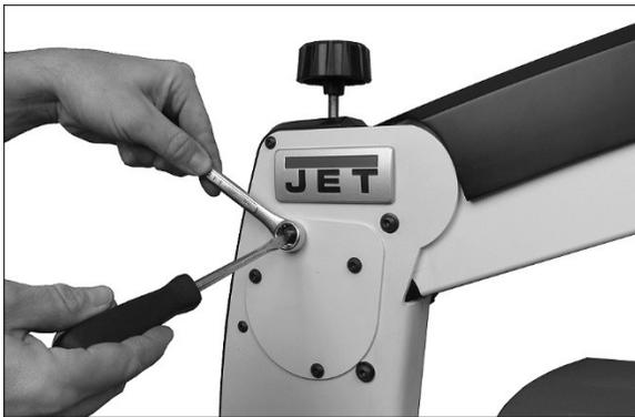
Figure 24: tightening arm lift
