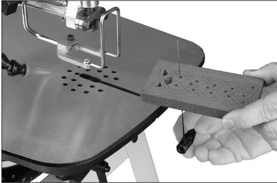
Figure 16: installing blade with workpiece
