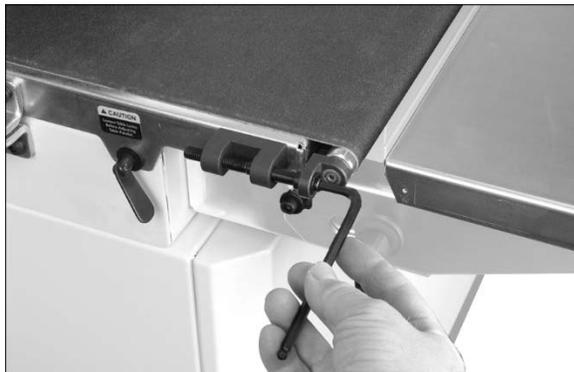
Figure 8-3: conveyor belt take-up screw
