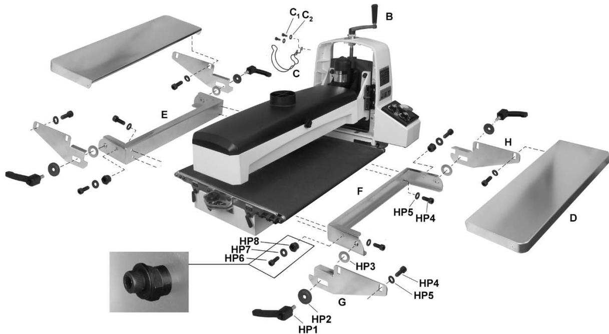
Figure 6-3: Assembly of Sander and OPTIONAL Infeed/Outfeed Tables
