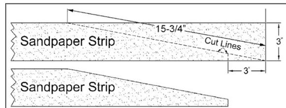
Figure 6-6: abrasive trimming
