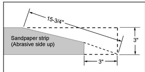
Figure 6-6: abrasive trimming – JWDS-1632 ONLY
