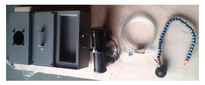
2. Take off the mid-cover from the coolant pump tank. The tank has pump and spray hose.
