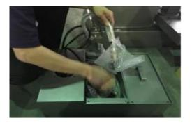
3. Install the coolant pump onto the top of tank, then put the mid-cover back to the original position.
