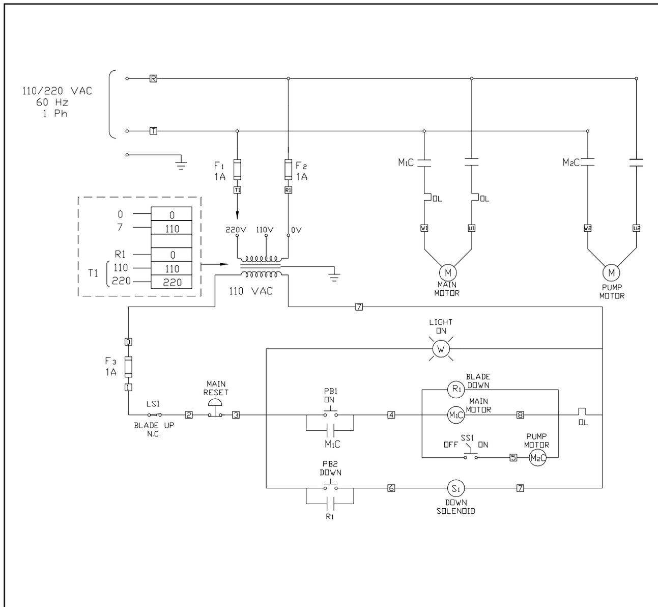
Figure 23: Model J-7020M cut-off saw wiring diagram
