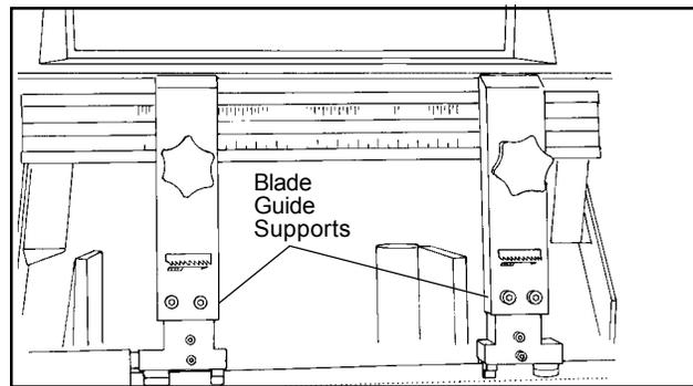
Figure 19: Blade guide supports
