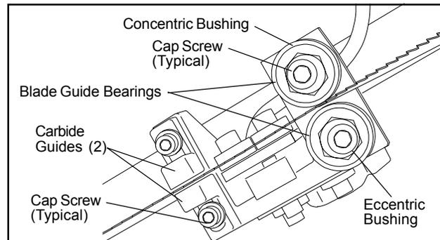
Figure 20: Carbide blade guides and guide bearings
