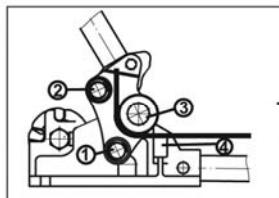
3. Open handle & insert rebar between 3 & 1,2 & 4.
