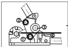
1. Open handle and insert rebar between 3 & 4 & 1.
