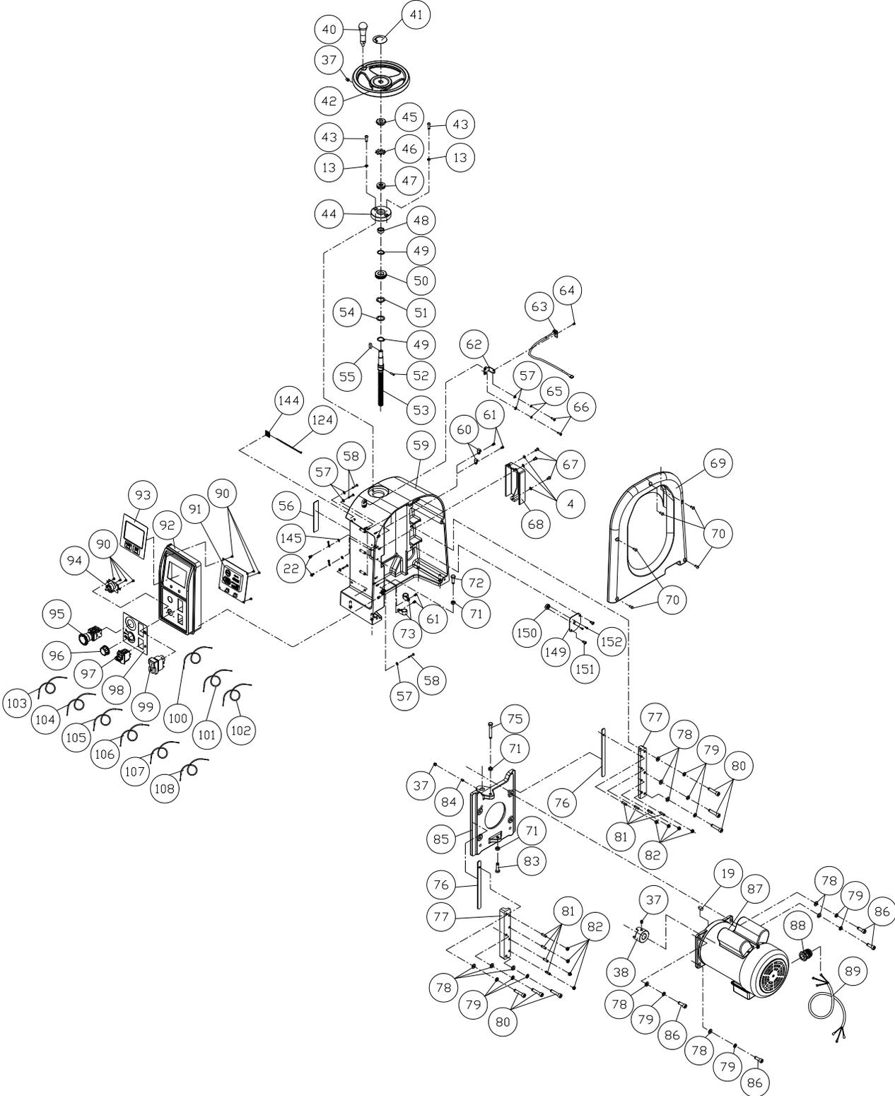
14.1.3 PM2244 Head Assembly III – Exploded View
