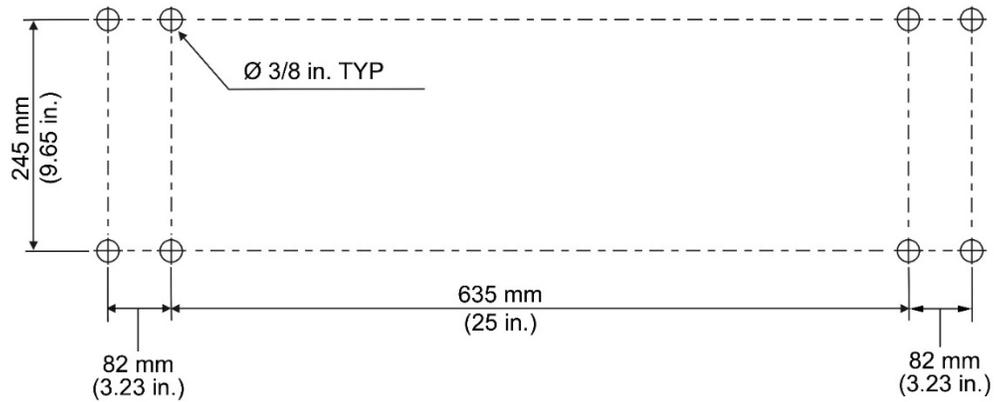
Figure 4-1: mounting pattern for workbench
