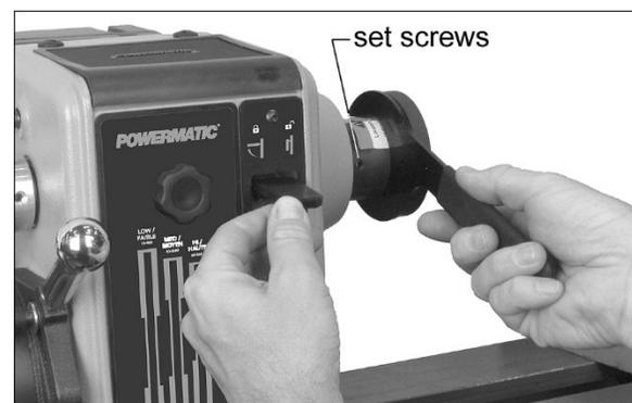
Figure 8-7: installing/removing faceplate
