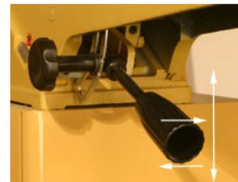
The infeed table height adjustments are truly unique. The handle can be moved up and down for coarse height changes or, after snugging the locking knob (to the left) the long handle can be rotated to make very fine, precise infeed table height adjustments.
