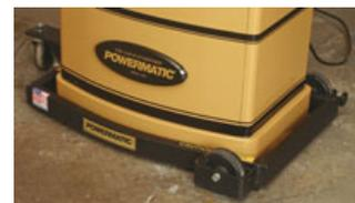
When you need to move the 54A/54HH joints around in your shop, our specially designed mobile base makes that an easy task.
