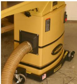
The all-steel base cabinet not only provides stable footing for the jointer, it houses the motor and dust collection outlet.
