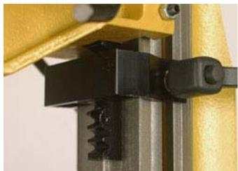
Mounting the depth stop directly
