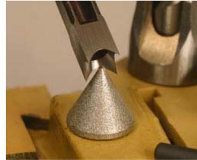
The special bushing spacer leaves (left) make setting the drill/chisel offset fast, easy and tool free. To keep the chisels sharp, a diamond encrusted sharpening point (right) is mounted on the column.
