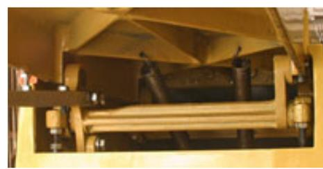
Both tables have easy to use handles (left) and locking knobs. The dual spring assist (right) makes these massive cast iron tables "feel" much lighter than they really are when making height adjustments.
