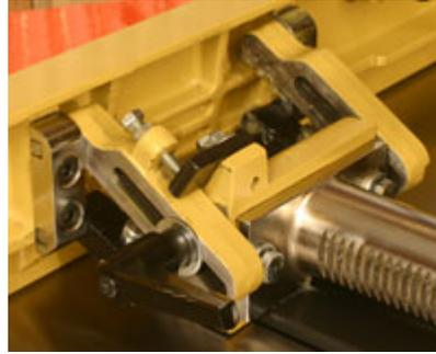
iron components that assure stability and truly accurate cuts at any angle. To insure flatness the face of the fence is surface ground.
