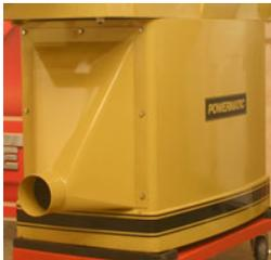
The all steel base cabinet houses the motor and the dust collection chute that terminates in a 4"-diameter port.
