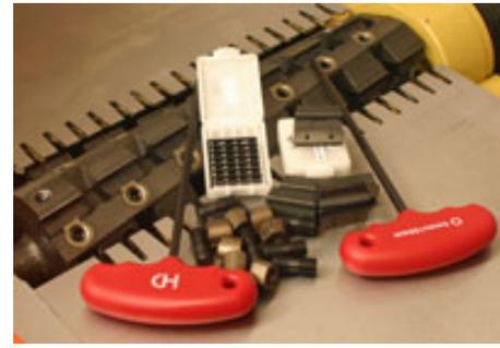
The helical inserts are easy to change because they are self-locating. (left) There is no shimming or adjusting needed. We include wrenches and spare inserts with mounting hardware (right) with the POWERMATIC 1285 Jointer.
