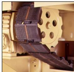
*Caterpillar feed blocks constructed of special grade cast iron are heat-treated and travel on special hardened and ground "V" ways. Auto oiler with shut off insures long trouble-free conveyor life. Variable feed speeds make it easy to get optimum feed/finish ratio.*
