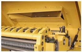
The large handwheel (left) makes raising and lowering the heavy cast iron table easy. The specially designed dust ports under the top cover (right) help evacuate the dust to keep the shop environment cleaner.
