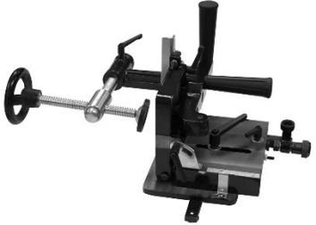
Figure 48 # 708295 – Tenoning Jig
