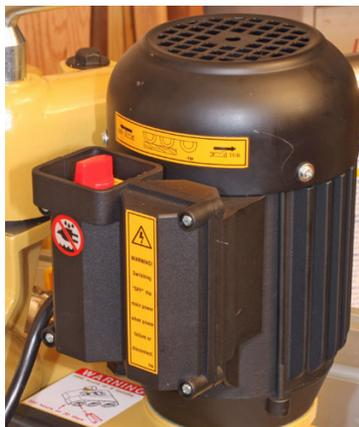
The powerful motor (left) has a tough cast iron case with integral cooling fins. The easy to change gear sets (right) included with the feeder provide four feed rates to fit any job.
