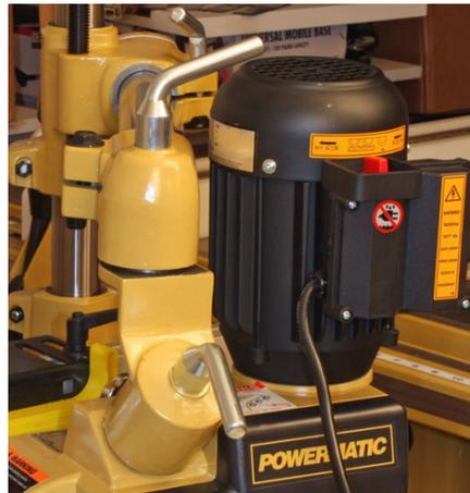
The column universal joints and cranks (left) make positioning the feeder very easy. The universal joints (right) make it easy to get the perfect feeder alignment or angle for the job easy.
