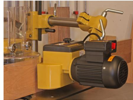
The articulated arms and universal joints allow using the Powermatic PF3-JR feeder to move stock flat on the table (left) or on edge at the shaper (right) for molding or face cuts.
