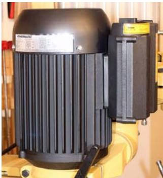
The powerful motor (left) is equally tough, starting with the cast iron case featuring integral cooling fins. Dual feed rates are easily accessed using the external control lever. (right)
