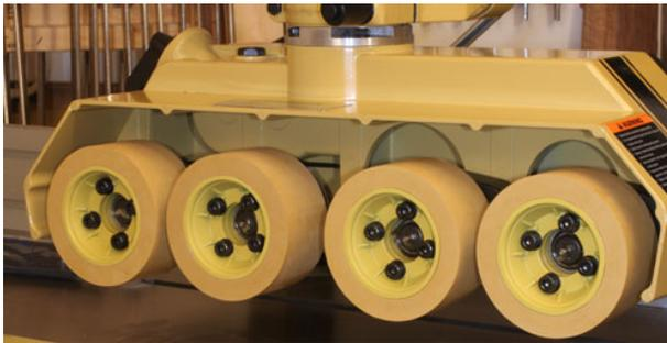
All four wheels (left) are mounted on individual suspension arms to insure a consistent, firm grip on the wood. Each wheel has a grease fitting at its center. The wheels are easy to change and can be replaced individually if needed.
