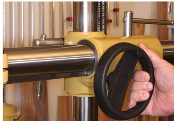
The support column (left) and arm (right) are made from heavy-walled steel tubing. Both have easy to use adjustments that make setting the PF-33 up for use simple.
