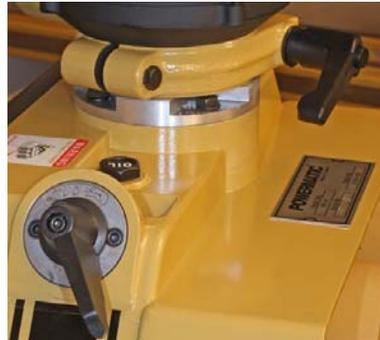
The POWERMATIC PF-31 Stock Feeder (#1790807K) is equipped with a heavy-duty 1 HP, 115 V (only), 1 Ph motor. The PF-33 is available with 230V (#1790800K) and 460V (#1790810K) 3 Ph motors.
