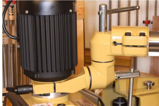
The mounting base (left) fits the twin mounting hole sets on the rear corners of the Powermatic PM2700 shaper but we include an easy to use bolt pattern template for mounting the PF-33 on other tools. The tool-free universal joints (right) make putting the PF-33 exactly where needed an easy task.
