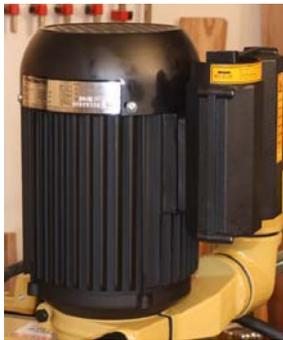
The PF-31 motor (left) is pure heavy-duty, starting with the cast iron case with integral cooling fins. The switch (lower right) on the feeder body selects the high and low speed ranges.
