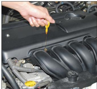
2. Select and insert the appropriate diameter extracting tube into the dipstick until it reaches the bottom of the oil pan, connect the main suction tube to the unit and to the extracting tube.
