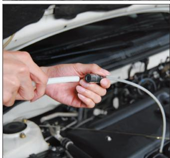
4. After all the oil has been extracted. Press the "Release Valve" for at least 5 seconds release any vacuum that may have formed in the inner pump tube. Remove the extracting tube from the dipstick tube (refit the oil dipstick). Remove the main suction tube from the unit. Slowly pour the used oil into a suitable container and dispose of it in an appropriate manner.
