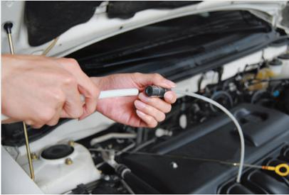
This Manual Fluid Extractor efficiently removes a variety of fluids from reservoirs on all types of vehicles and equipment. The manual pump vacuum operation eliminates the need for compressed air making it portable and versatile. Extract fluids through filler ports and dipstick tubes using the included extractor tubes.
