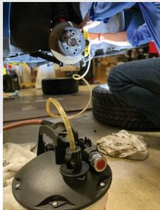
Removing and replacing fluid is now a one-person job. This Pneumatic Brake Fluid Exchanger makes brake bleeding clean and simple using compressed air and a venturi vacuum system. Use to evacuate a variety of other fluids from vehicles or small engines. Includes a bleeding tube and fluid refill bottle.
