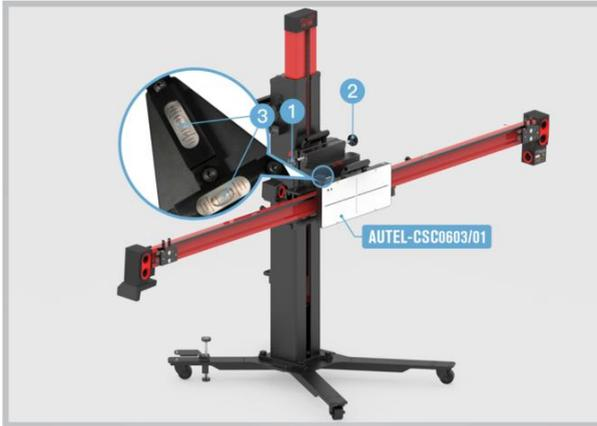
2. Plug the included power cord into the power port (1). Turn on the power switch (2) and the red LED (3) will light up.
