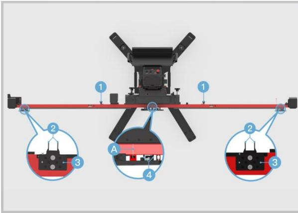
5. Loosen the handle (1) and rotate the fine-tuning bolt (2) until the position A is aligned with the red marked line. Tighten the handle (1) to secure the crossbar.
