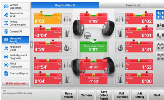
**Figure 5-85 Measured Result (Half Tolerance) Screen**
