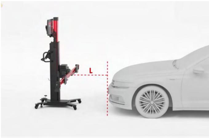
**Figure 6-64 Center the Calibration Frame**
