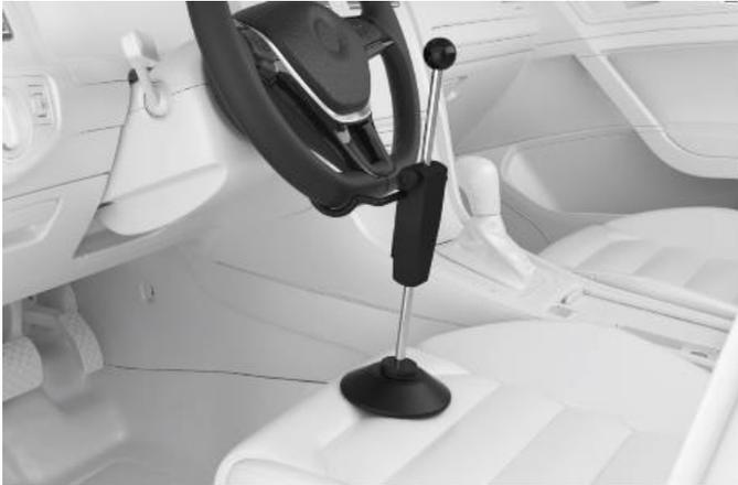
**Figure 6-147 Install the Steering Wheel Holder Stand Tool**
