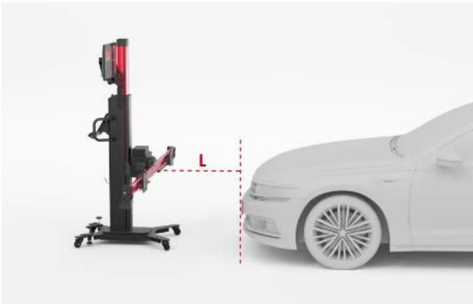
**Figure 6-77 Center the Calibration Frame**
