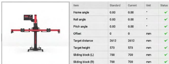
**Figure 6-51 Move the Crossbar to the Target Position**
