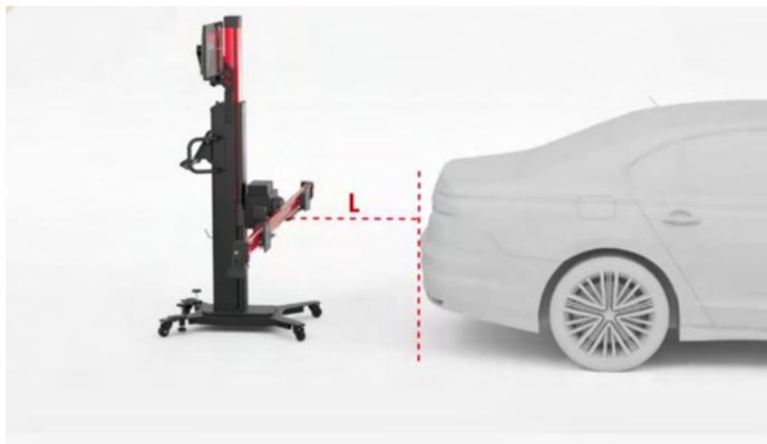
**Figure 6-30 Center the Calibration Frame**
