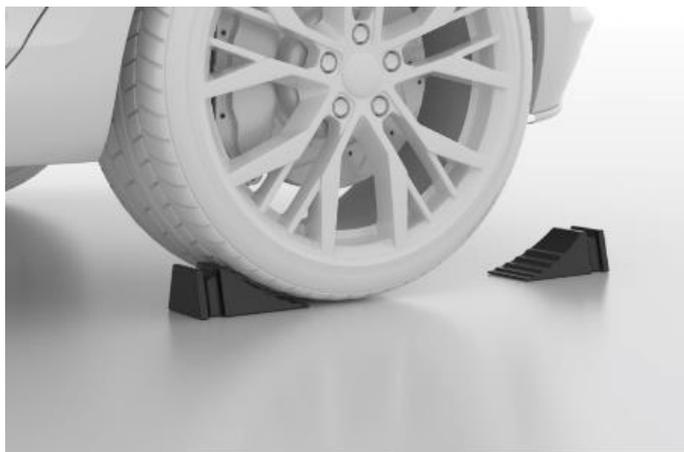
**Figure 6-75 Place the Wheel Chocks**
