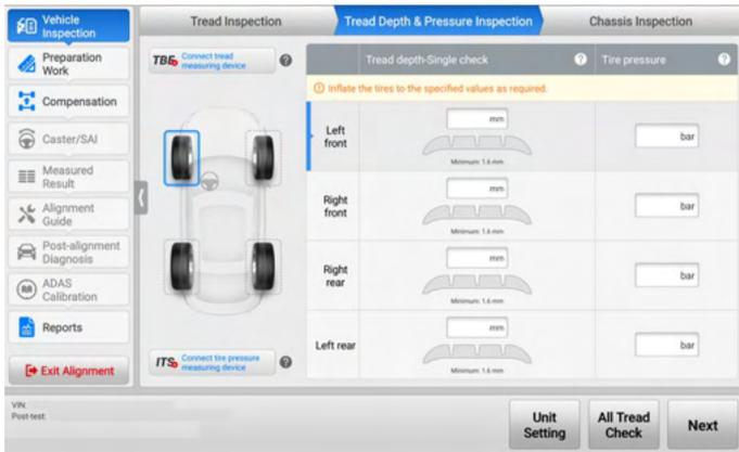
**Figure 4-15 Tread Depth & Pressure Inspection Screen 1**
