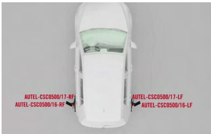
**Figure 6-31 Install the Wheel Clamps (Tire Clamps) And Targets**
