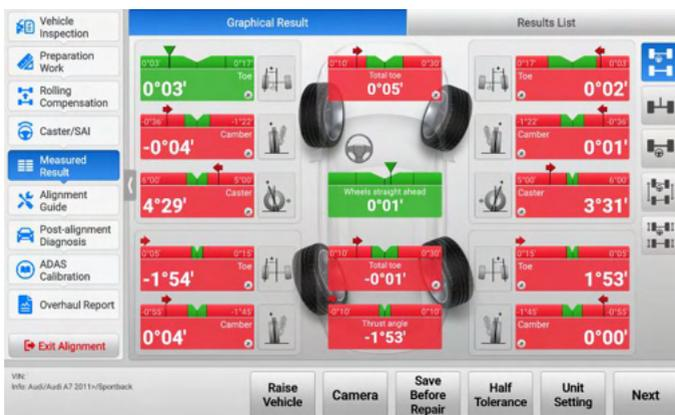
**Figure 5-86 Measured Result (Full Tolerance) Screen**
