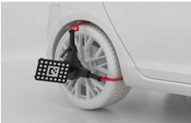
**Figure 6-137 Install the Wheel Clamps (Tire Clamps) And Targets**
