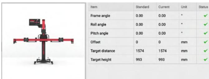
**Figure 6-157 Move the Crossbar to the Target Position**
