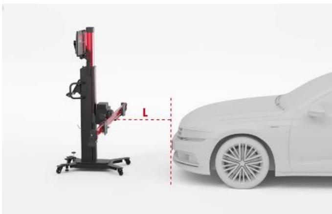
**Figure 6-108 Center the Calibration Frame**
