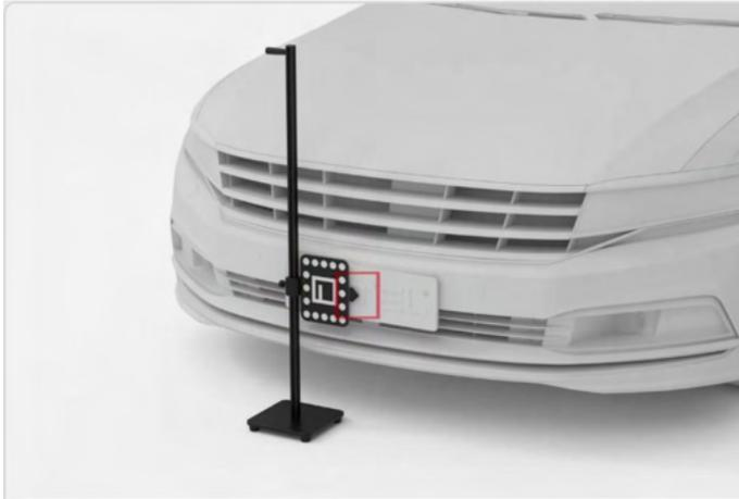
**Figure 6-97 Place the Alignment Aid**
