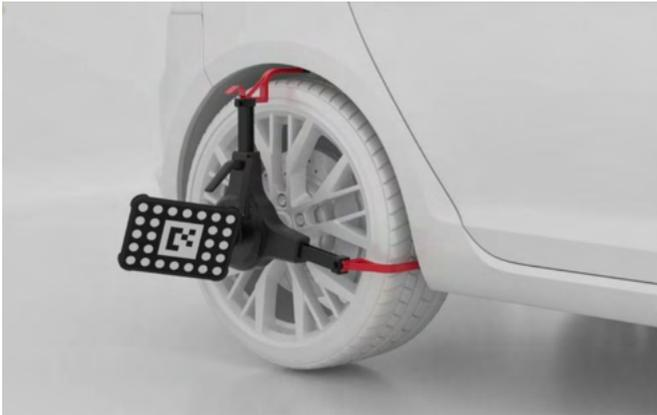
**Figure 6-122 Install the Wheel Clamps (Tire Clamps) And Targets**
