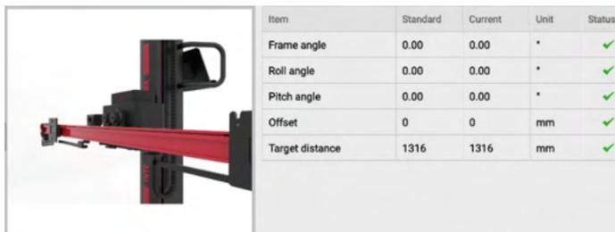
**Figure 6-113 Move the Crossbar to the Target Position**
