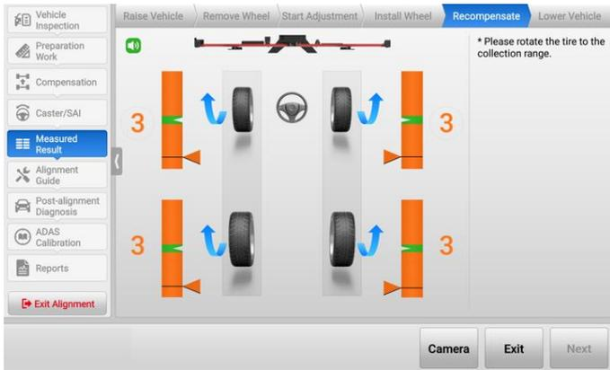
**Figure 4-57 Start Lifting Compensation 2**
