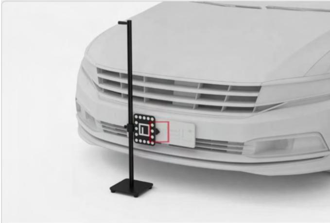
**Figure 6-123 Place the Alignment Aid**
