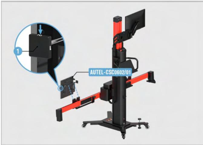
**Figure 6-17 Adjust the Reflector 1**
