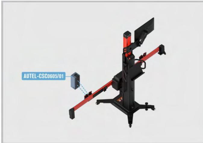
**Figure 6-34 Install the radar calibration box on the Left Sliding Plate**
