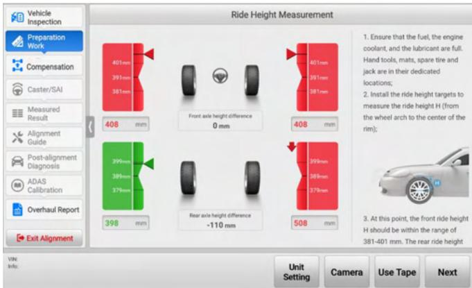
**Figure 4-33 Measure Ride Height with Ride Height Target**
