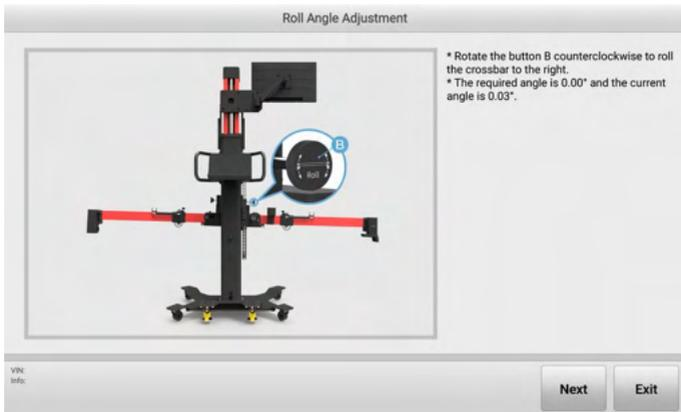
**Figure 5-64 Roll Angle Adjustment 2**
