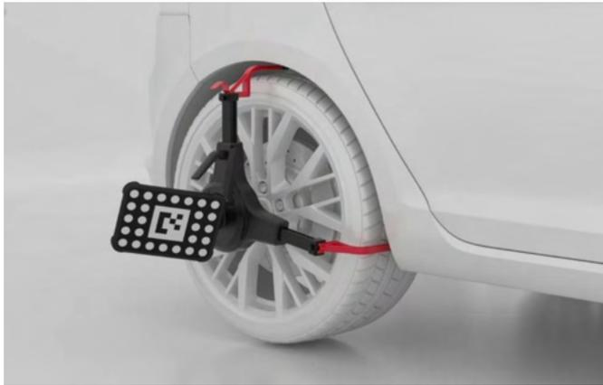
**Figure 6-109 Install the Wheel Clamps (Tire Clamps) And Targets**
