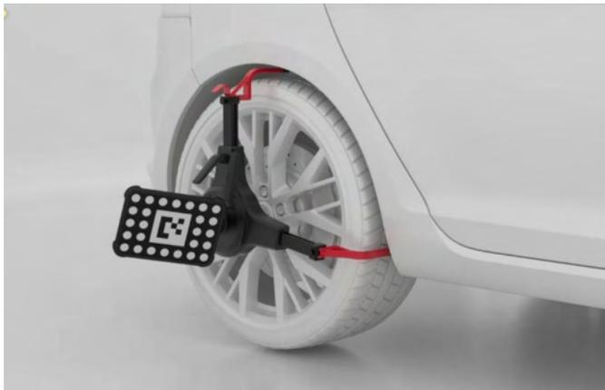
**Figure 6-149 Install Wheel Clamps (Tire Clamps) And Targets**
