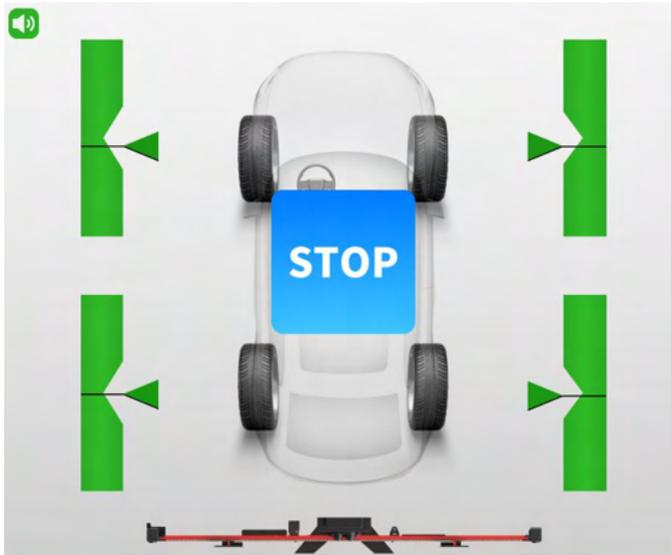
Figure 6-47 *Wheel Rolling Compensation 2*
