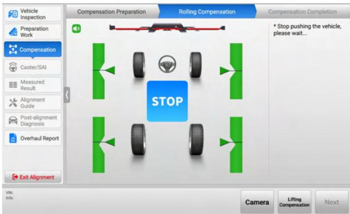
**Figure 4-39 Start Rolling Compensation 4 (Use Tire Clamp)**
