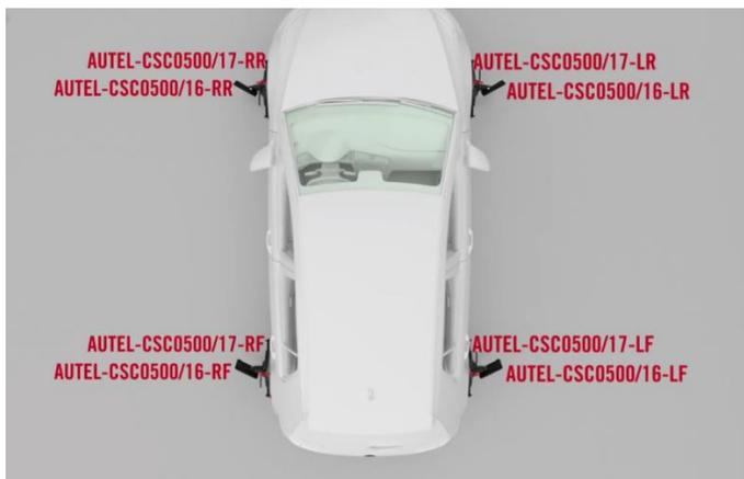
**Figure 6-45 Install Wheel Clamps (Tire Clamps) And Targets**
