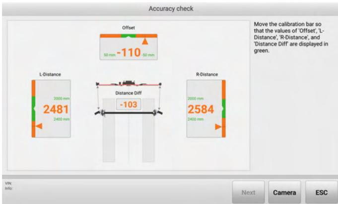
**Figure 5-41 Accuracy Check Screen (Use Calibration Bar) 2**
