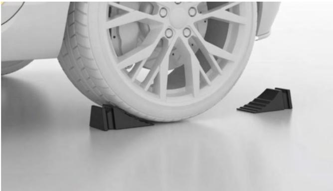
**Figure 6-42 Place the Wheel Chocks**
