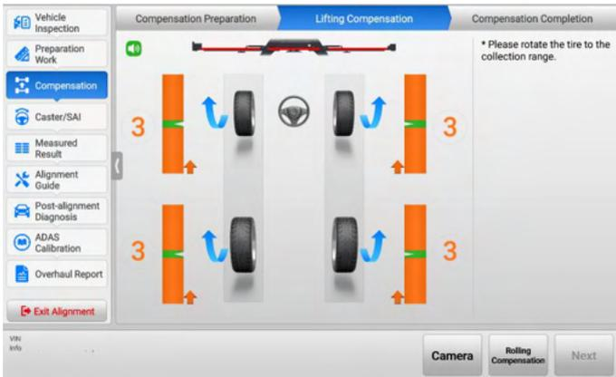
**Figure 4-43 Start Lifting Compensation 2 (Use Tire Clamp)**
