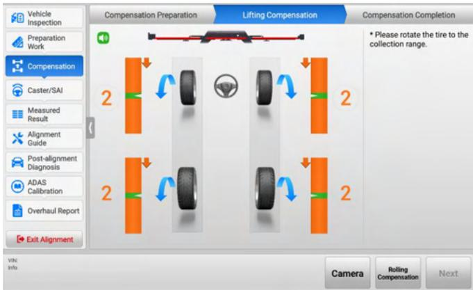
**Figure 4-44 Start Lifting Compensation 3 (Use Tire Clamp)**
