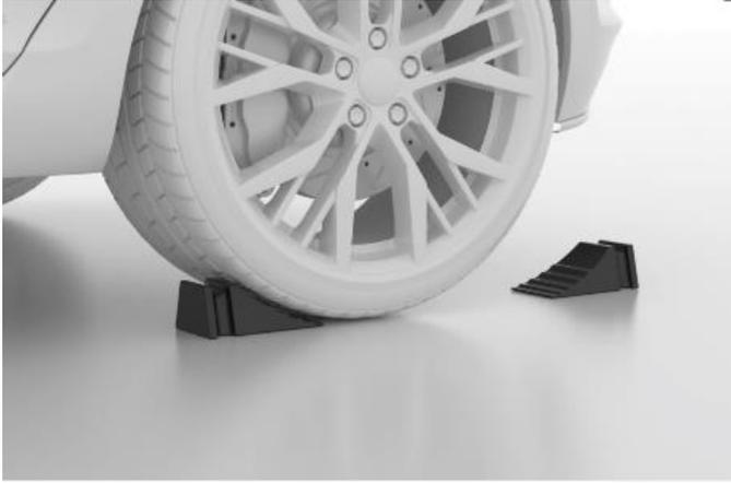
**Figure 6-146 Place the Wheel Chocks**
