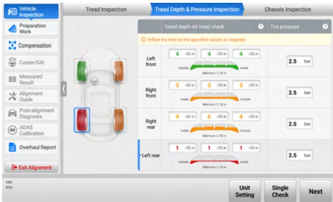
**Figure 4-19 Tread Depth & Pressure Inspection Screen 2**
