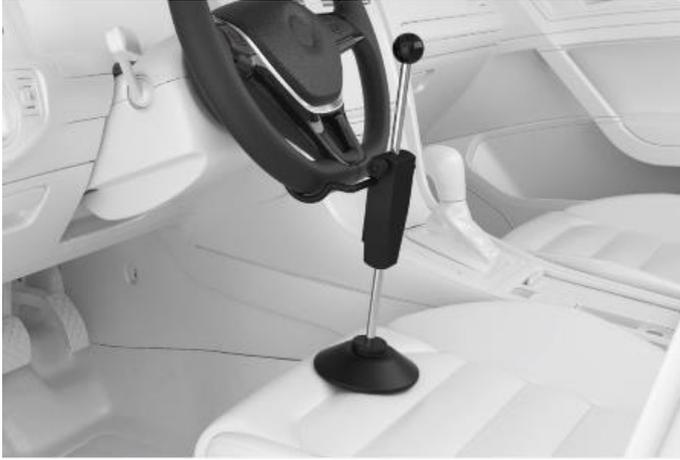
**Figure 6-76 Install the Steering Wheel Holder Stand Tool**
