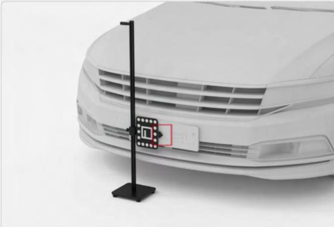
**Figure 6-5 Place the Alignment Aid**
