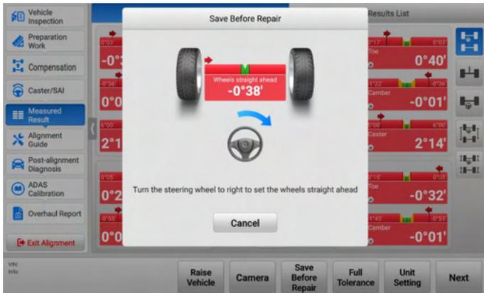
**Figure 5-83 Save Before Repair Screen 1**
