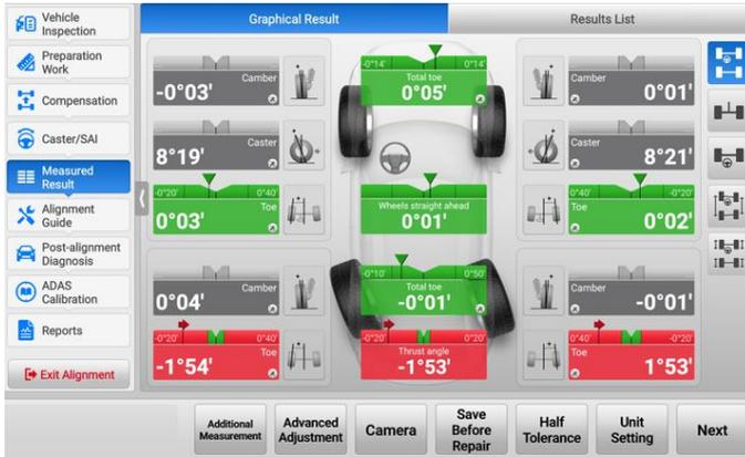
Figure 4-48 Measured Result Screen (Graphical Result)
