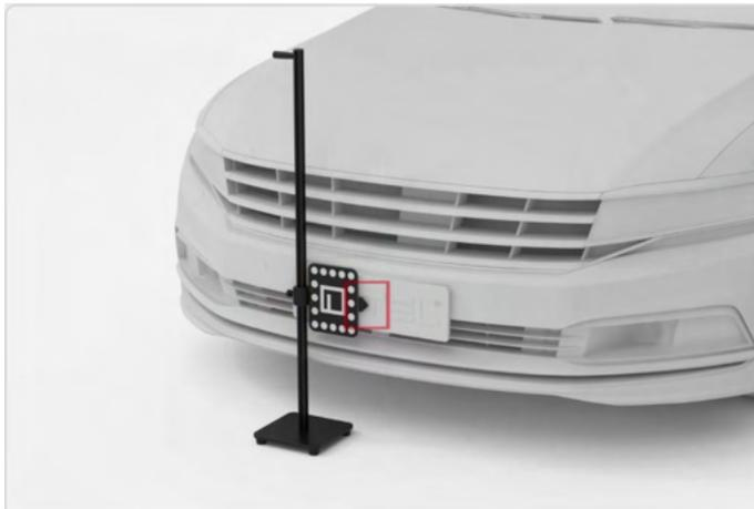
**Figure 6-110 Place the Alignment Aid**
