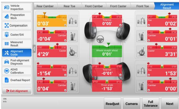
**Figure 4-64 Alignment Result Screen**
