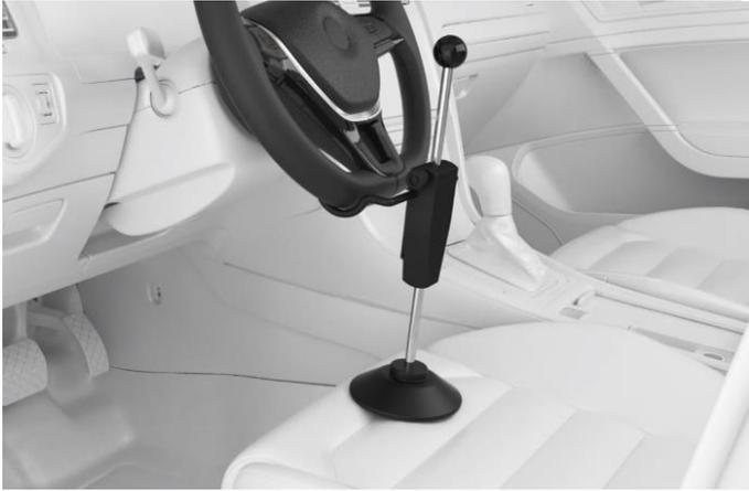
**Figure 6-43 Install the Steering Wheel Holder Stand Tool**
