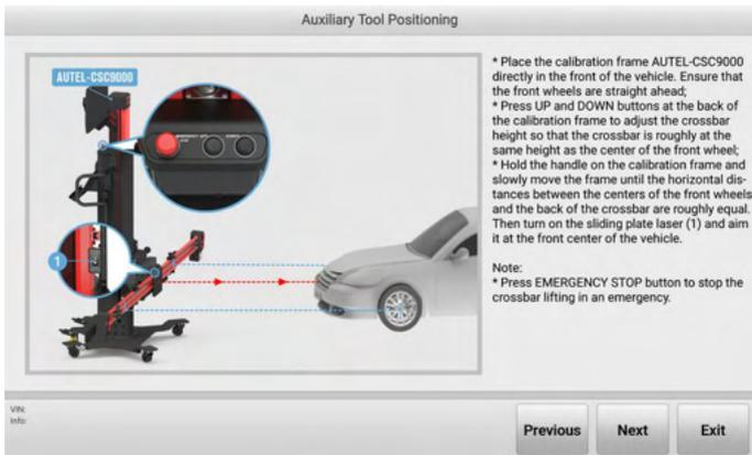
**Figure 5-58 Auxiliary Tool Positioning 3**
