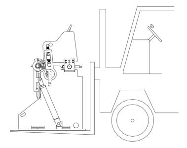
2. Installation: When installing machine should be installed in a horizontal on the bottom of foundation, level the machine very well, using leveling pads or foundation bolts.
