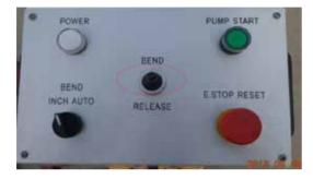
e. On the auto bending mode, turn the mode selection switch to inch, press and hold the unclamp foot pedal to raise the upper beam, insert the material, and press and hold the clamp foot pedal to clamp the material tightly. Then press and hold the BEND foot pedal, the bending leaf lifts up, bend the material, and return back down to the bottom position, make one cycle bend.
