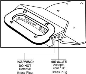
Add a few drops of pneumatic tool oil to air inlet occasionally (monthly).
