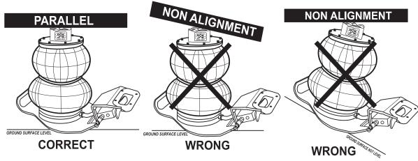
WARNING: RAK JAK base and lifting surface should always be parallel to jack to avoid jack from slipping. NON ALIGNMENT MAY RESULT IN LOAD DROPPING SUDDENLY, WHICH MAY CAUSE SEVERE INJURY OR DEATH.
