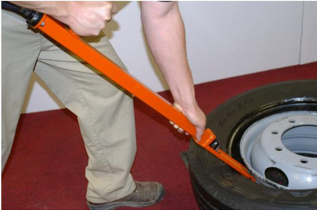
**Place tool at an approximately 45 degree angle and insert between 2nd tire bead and rim.**
