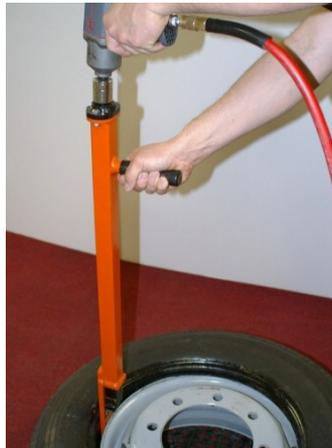
**When the first bead is removed, turn the impact tool in a clockwise motion to reset the pushing arm.**
