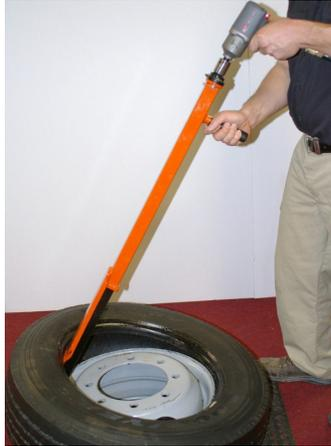
**Begin to extend the push foot with an impact wrench in a counter clockwise motion. As the pushing foot begins to meet the rim, ensure that the plastic protective angle properly engages the rim edge and allow the natural motion of the tool to rock backwards.**
