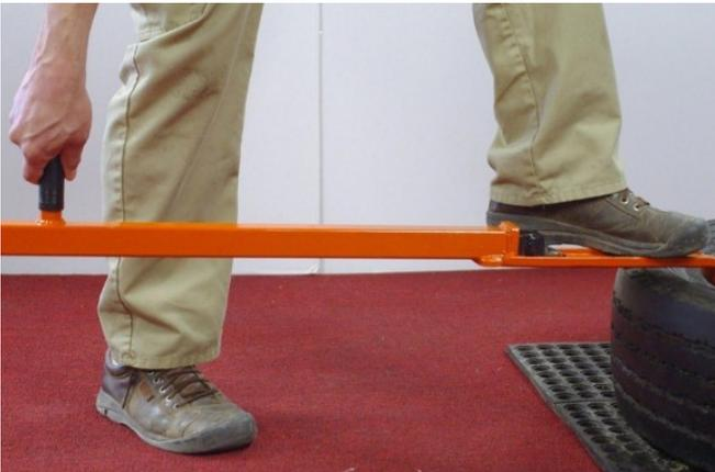
**Insert the tool between the rim and tire bead by laying the tool horizontal and using downward pressure with your foot until the heel of the pulling foot is below the plain of the rim.**
