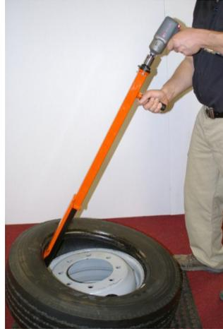
**Continue to retract the pulling foot with the impact wrench while bringing the tool towards the wheel center in a pivoting motion until the 1st bead is removed. NOTE: Do not force or excessively pry with the tool. Allow the natural motion of the pulling foot to remove the tire.**
