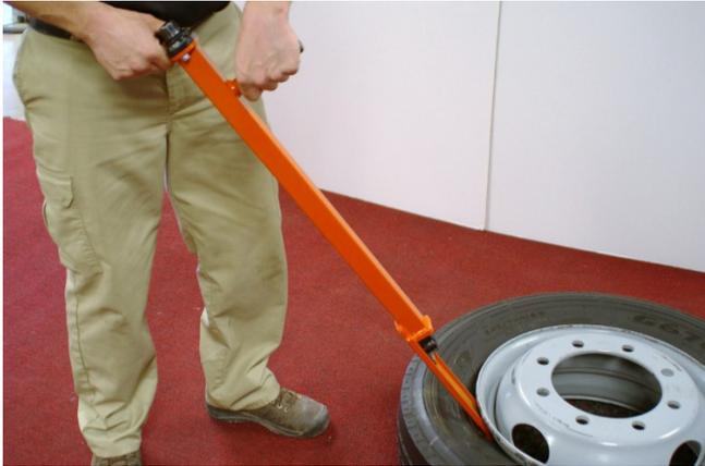
**Bring tool to an upright position to engage the puller foot between rim and inside tire bead.**
