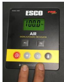
The display screen will show a reading of “**100 PSI**”, at this point shut off the air source and calibration is complete.
