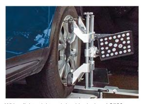
With a lightweight and durable design, AC700 clamps have the capacity to easily accommodate rims that range from 11"-22".
