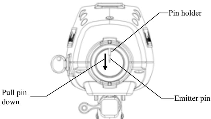
5. Insert the new emitter pin using the tweezers or pliers. Be sure to push the emitter pin in as far as it will go.
