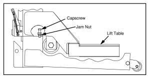
Fig. 10: Lift table clearance adjustment
