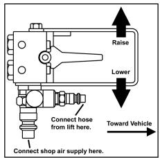
Fig. 3: Air control lever
