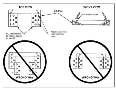
Fig. 11: Installing the WL-adapters
