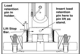
Fig. 6: Load retention pin
