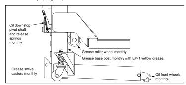
Fig. 8: Lubrication points
