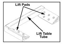
Fig. 12: Lift table tube identification
