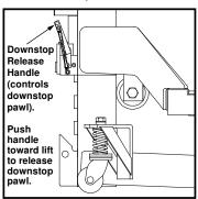
Fig. 7: Push downstop release handle torward lift
