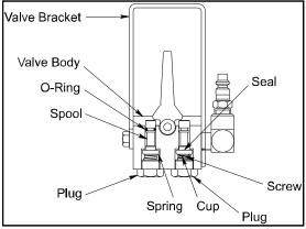
Fig. 9: Air control unit component identification
