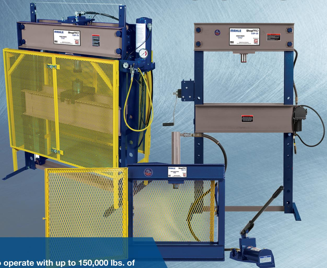
Able to operate with up to 150,000 lbs. of available pressure to be applied to any part that requires a consistent force to remove or replace.
