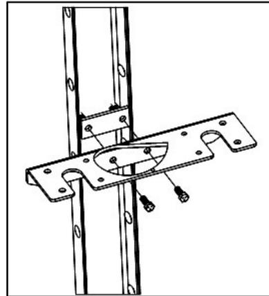
Fig. 6: Attaching pump bracket
