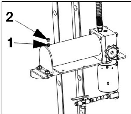
Fig. 9: Installing breather vent plug
