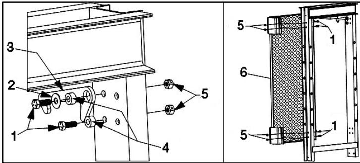
Fig. 13: Guard installation
