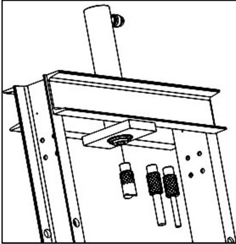
Fig. 11: Remove cap to install pushing adapter
