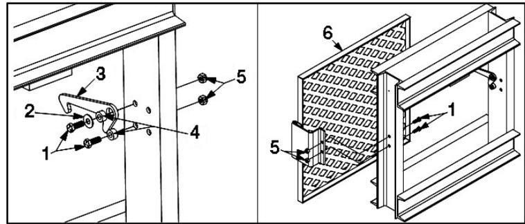
Fig. 14: Guard installation
