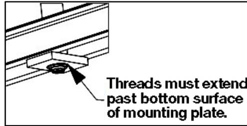
Fig. 5: Installing hydraulic cylinder
