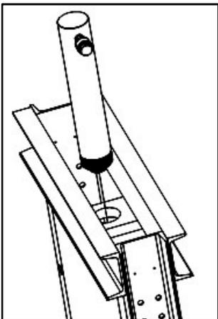
Fig. 4: Thread cylinder into mounting plate
