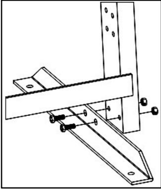
Fig. 3: Install support feet
