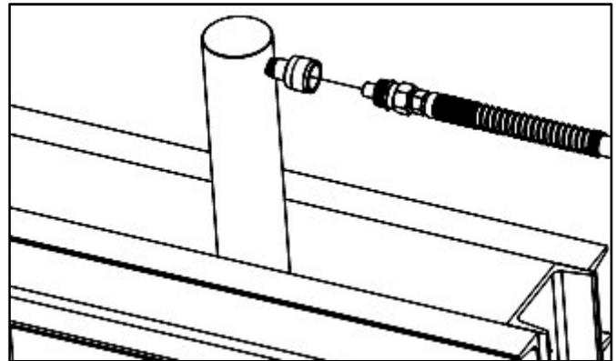
Fig. 10: Connecting hydraulic hose
