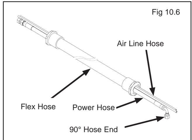
6. Install the end of Flex Hose with the Straight Fitting on the Hydraulic Hose into the hole in the Powerside Runway adjacent to the Power Unit. Install the end of the Flex Hose with the 90° Fitting on the Hydraulic Hose in the Flex Hose Bracket Assy. Tighten the plastic nuts securely. (See Fig 10.7)
