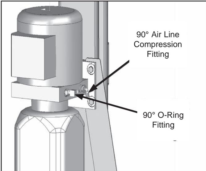
2. Remove the captive nut on the Compression Fitting. Insert the Plastic Air line through the alignment sleeve and into the end of the fitting until it bottoms out. Then tighten the nut on the fitting. (See Fig 10.3)
