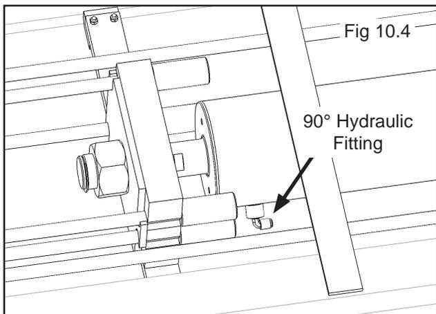
4. Install the 90-degree Air Line Compression Fitting in the port at the base, pinned end of the Cylinder. On the pipe thread side of the Fitting, it is recommended to use Teflon Tape or pipe sealer. (See Fig. 10.5)
