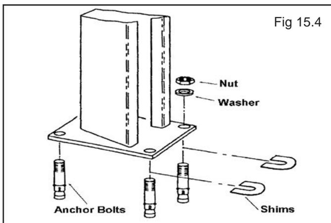
6. After any necessary shims are installed, tighten each nut to 35-45 ft./lbs. **IMPORTANT** - If Anchor Bolts do not hold when torqued to required amount, concrete must be replaced. Saw cut and remove 24" x 24" square area each Column base then re-pour with reinforced 2500 concrete to a depth of six inches minimum, keying new concrete under existing floor. (See Fig. 15.5)
