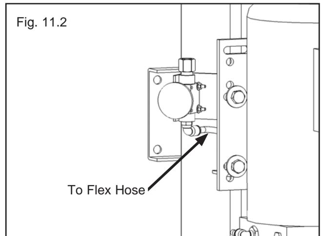
3. Once the air line has been connected with the Push Button Air Valve, cut the air lines to length by following the Safety Air Line Routing diagram located on Page 25 and connect female branch “tee” fittings where needed.
