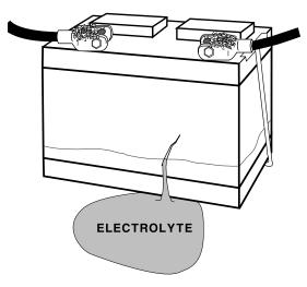
Important Note: A damaged battery must be replaced before proceeding.
