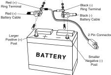
**NOTE:** Smaller batteries may have screws for terminals (see illustration below). You may need to purchase smaller ring terminals for these applications. Do not connect ring terminals to anything but the battery. Other locations are hazardous.
