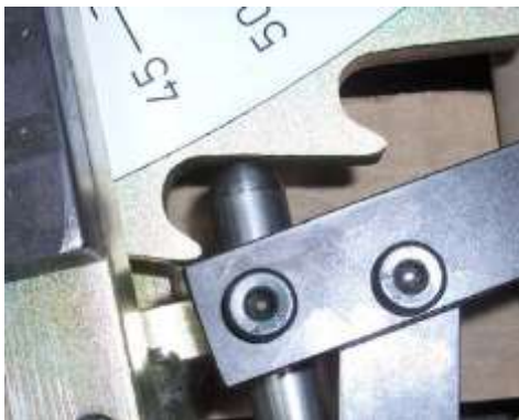
Anti-springback lever engaged
