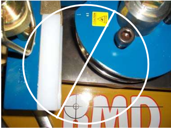
Too far away from die
