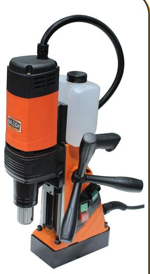
*IMPORTANT:* The drill's magnetic adhesion depends on the thickness of the work piece. 0.59" – 1.96" (15 – 50mm) is optimum thickness for safe operation. If the material is less than 0.59" (15mm) thick, the material may not produce enough magnetic adhesion. In some cases, adding a backer plate under the magnet on the back side of the work piece may
