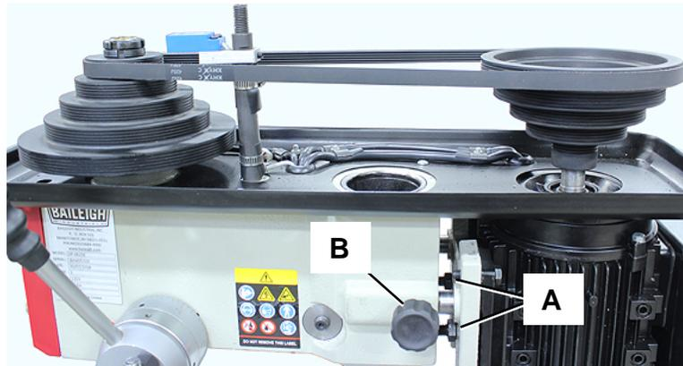
6. Loosen the tension lock knobs (B, one on each side of head) and allow the motor to slide slightly closer to the spindle. This will loosen the belt enough to allow it to be moved to another set of pulleys.
