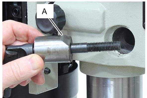
**⚠ CAUTION:** Before operating the drill each day, verify that the head is secured to the column. Failure to ensure that the head is secure to the column may allow the head to twist unexpectedly during operation causing damage and or injury.
